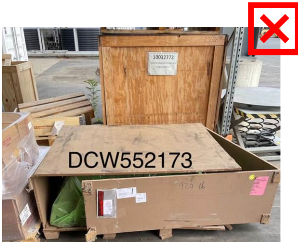
Insufficient strength/design crate packaging used to transport heavy metal components. Crate collapsed during movement presenting a safety risk and damage to goods.
