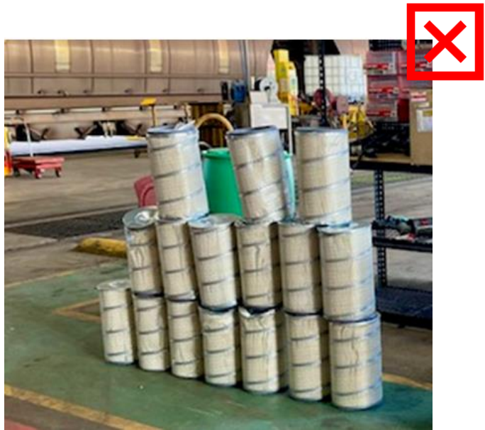
Goods placed horizontally within palletised consignment sustaining extensive damage as the result of double staking. No “No double stacking” labelling applied, PTE strapping or corners used to secure the load. Pallet wrapping was applied too tightly causing it to tear. Damaged filters were not received.
