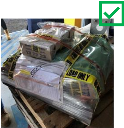
Examples of correct pallet loads with goods secured using PTE strapping and corners, and then unitised to a pallet using clear wrapping. Pallet top cover used to ensure good weather protection. Labelling clearly visible to prevent possible goods damage during transit from stacking.
