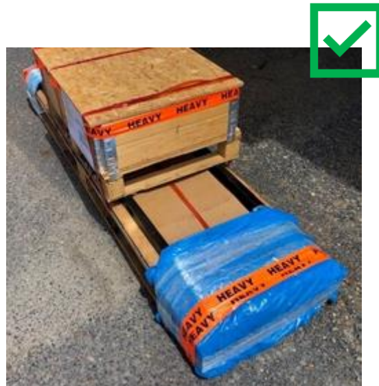
Oversized goods secured to a custom wooden pallet using PTE strapping. Wooden crate location is centrally positioned to balance the load. Clear labelling is used to label consignment as 'Heavy'.
