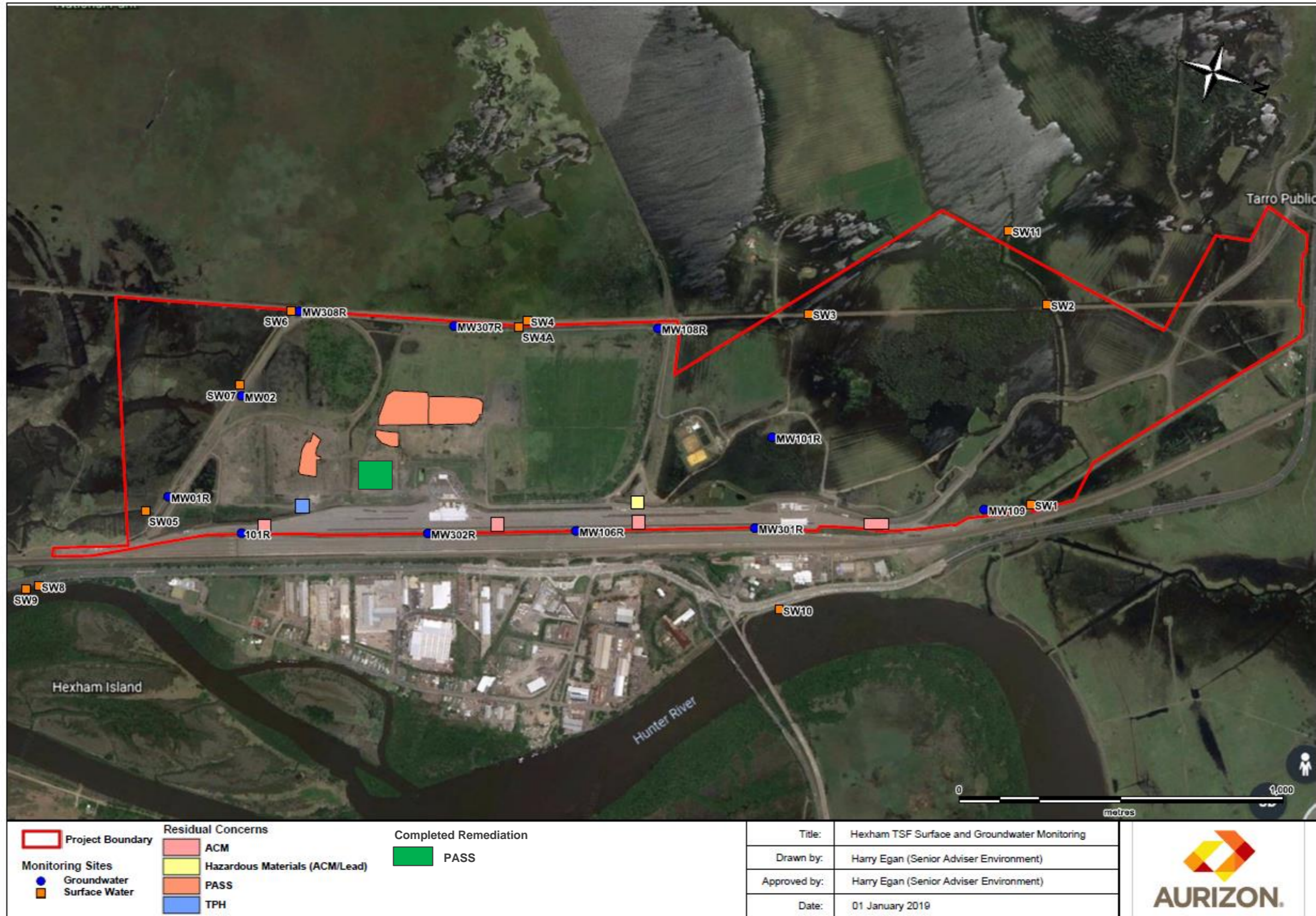
Figure 3 – Hexham TSF Environmental Monitoring Network
