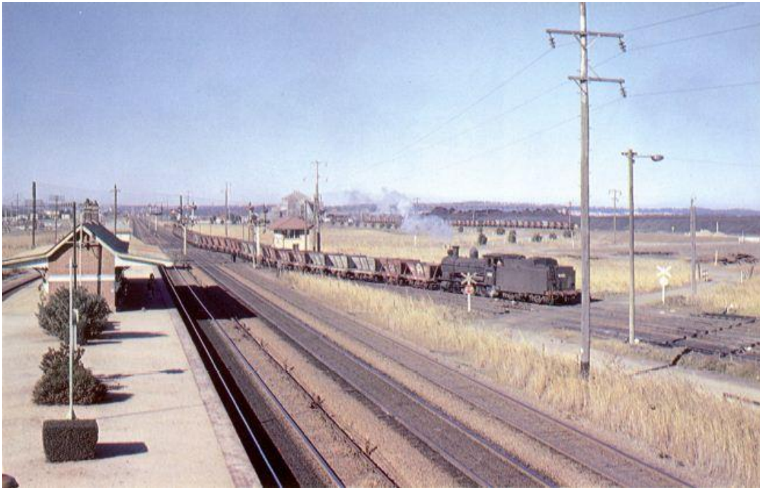
Figure 21. A NSWGR 'Standard Goods' engine leads its train into the Hexham exchange sidings. The station and signal box, both now demolished, are shown. The Coal Preparation Plant and its sidings are in the middle distance. The Late Ron Preston
