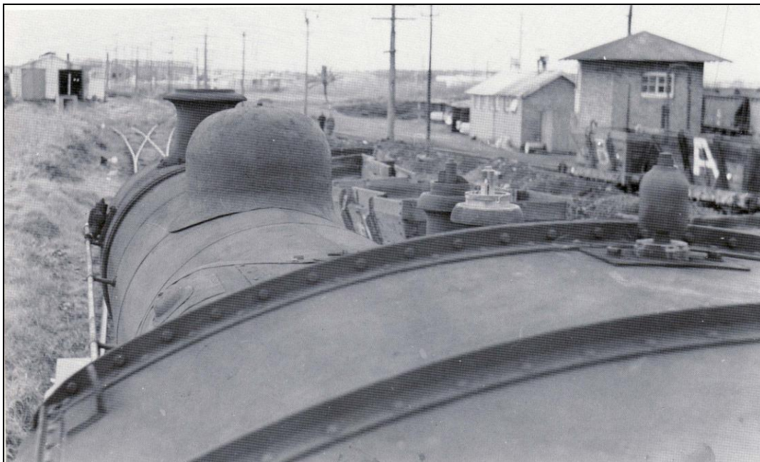
Figure 17. View from the tender of an R.O.D. locomotive stored in the former crushing plant sidings. Note the engine shed, Bath House and Control Cabin. The government steel bogie wagons seen to the right of the Control Cabin are unusual intruders in the maze of non-air braked four-wheeled hopper wagons. The Late Ron Preston
