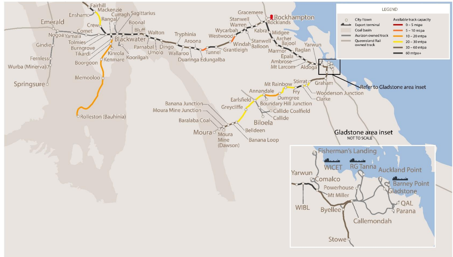
Figure 4: Blackwater and Moura System available capacity and constraints
