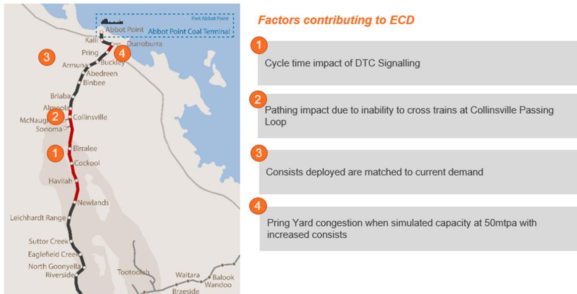
The ICAR indicates that the constraining section for both the Newlands and GAPE Systems is the branch line between Pring and Newlands Junction. Aurizon Network's review has isolated specific operational factors within this section that are the contributing to this constraint:
