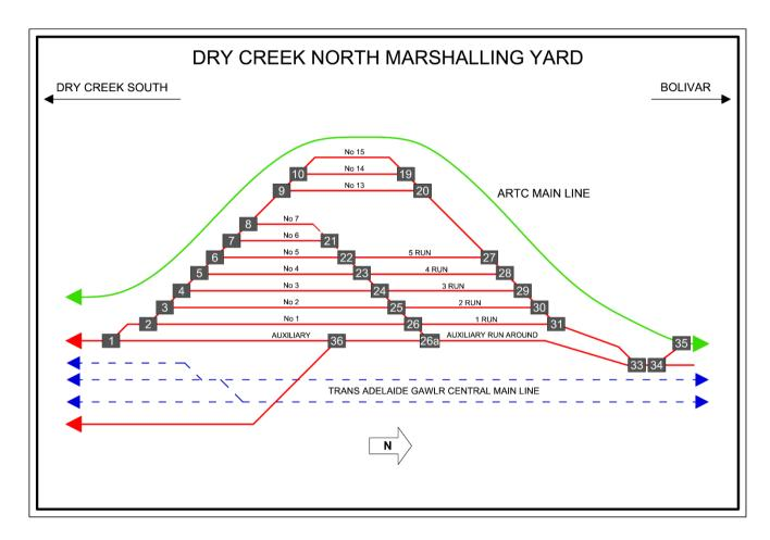
Clear standing room in the Dry Creek North Marshalling Yard (Standard Gauge) is as follows:
